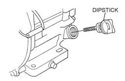
Figure 15. Engine Oil Dipstick (Removal)
